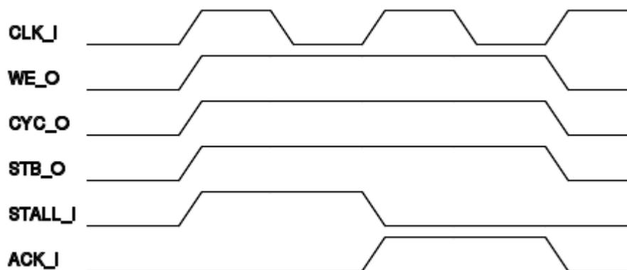
*Illustration 5-1: Write - pipelined master standard slave*
