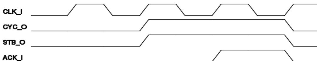
Illustration 3-3: Standard wishbone handshaking protocol, synchronous slave.
