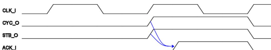
*Illustration 3-2: Standard bus handshaking protocol, asynchronous slave.*
