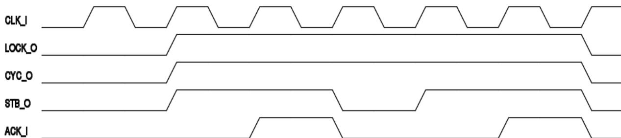
*Illustration 3-9: Use of [CYC\_O] signal during BLOCK cycles*
