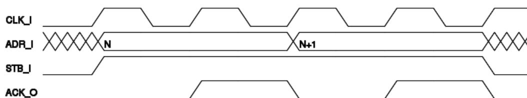
Illustration 4-2: WISHBONE Classic synchronous cycle terminated burst
