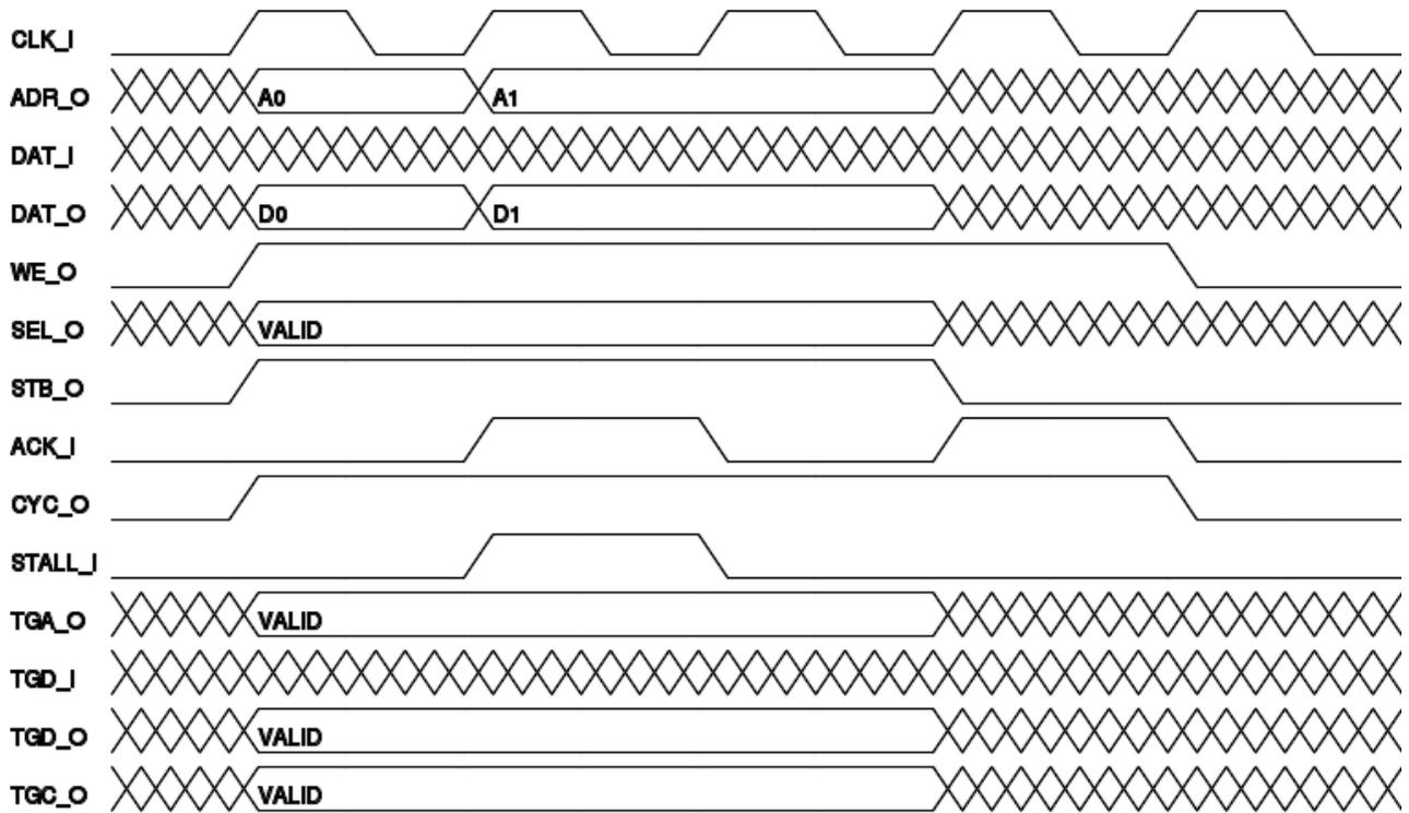
*Illustration 3-13: Pipelined BLOCK WRITE cycle*
