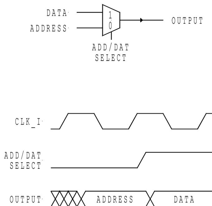
Illustration 8-17: Circuit and timing diagram for a multiplexed address/data bus
