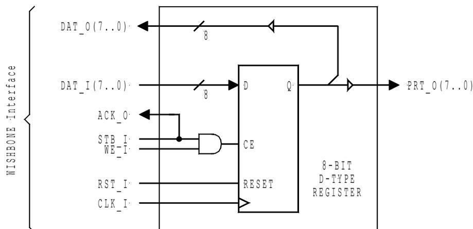
Illustration 8-9: Simple 8-bit WISHBONE SLAVE output port
