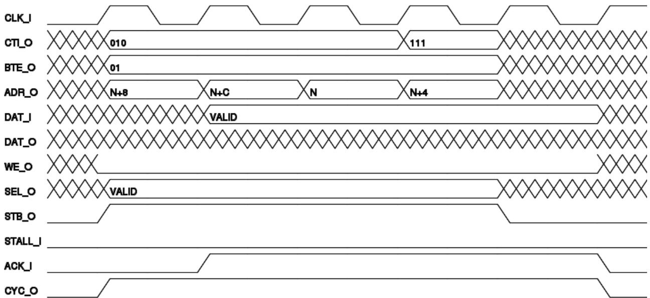
*Illustration 4-11: 4-beat wrapped incrementing burst for a 32bit data array, pipelined*
