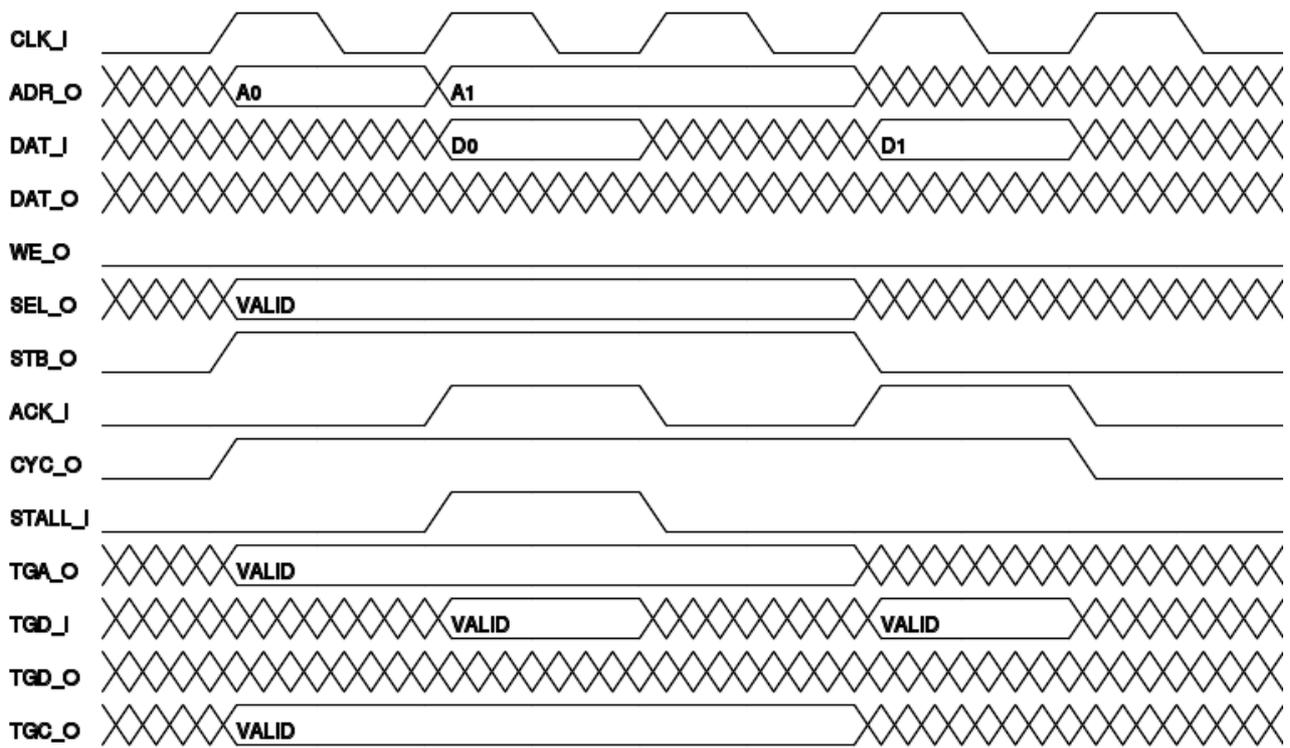
*Illustration 3-11: Pipelined B4 BLOCK READ cycle*
