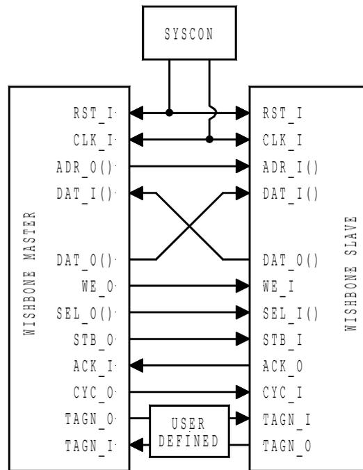
*Illustration 1-2: Standard connection for timing diagrams.*
